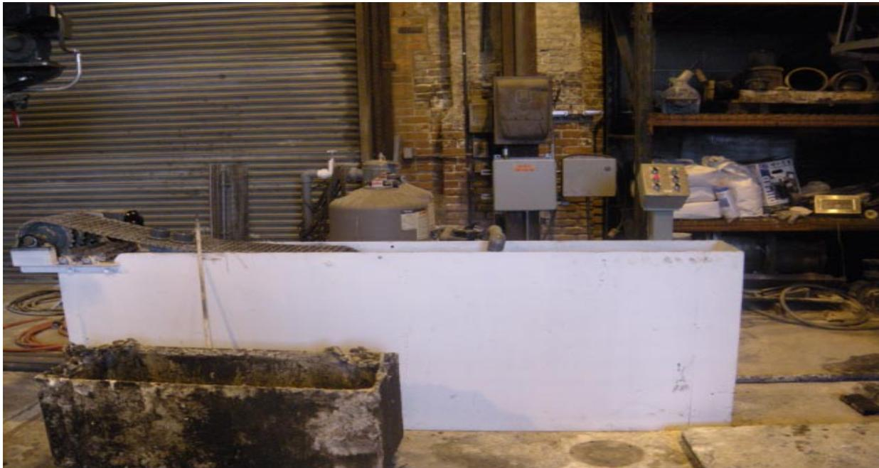
**(13) Solids Recovery Reservoirs** – Solids and fines from the PSV and filters are collected and weighed here ready for landfill. If a solids filtration and washing stage is of interest to the user, it would be placed between here and the PSV.
